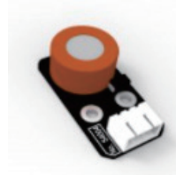
▲ Gas leak sensor
