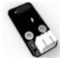
Earthquake sensed using a tilt sensor
