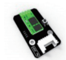
Related data sent to smartphone or warning device via bluetooth
